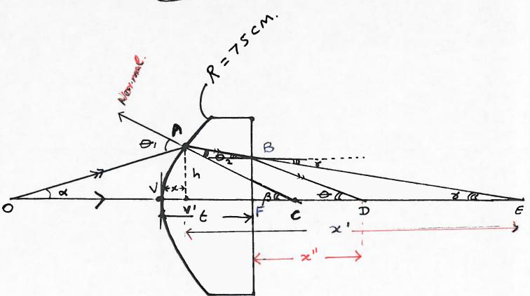
The Ray diagram is as shown. The Image is oneated at D. "C" is the centre of the curved San face. ... AC is a Normal to the curved sample.
